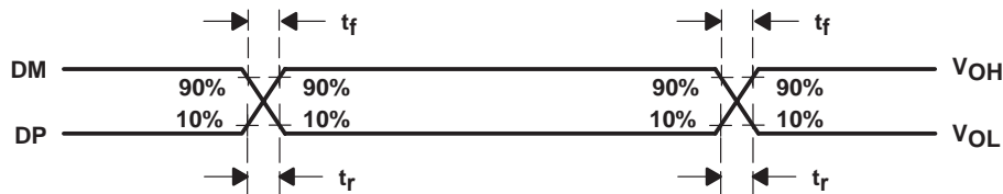
Figure 1. Differential Driver Switching Load
