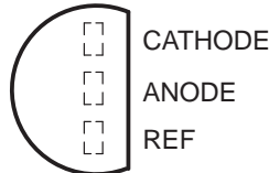
TLVH431 LP (TO-92/TO-226) PACKAGE (TOP VIEW)
