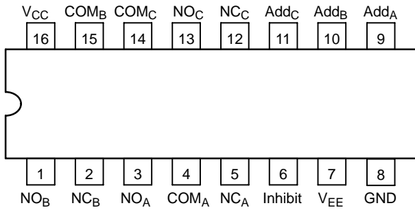
Figure 1. Pin Connection (Top View)
